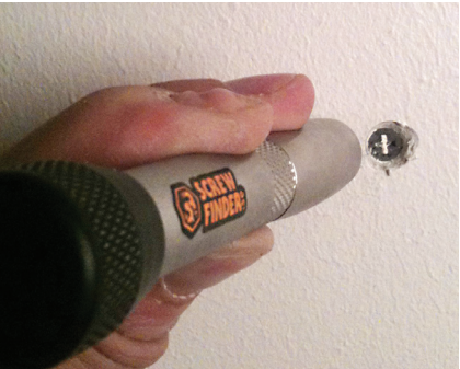
MARK LIGHTLY WITH A HAMMER WHEN SCREWFINDER FINDS THE SCREW. THE SCREW IS EXPOSED.
